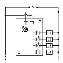
SC4 shown; for SC3, terminal 6 & load L4 are eliminated.
