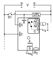
S1 = Initiate Switch L = Timed Load UTL = Untimed Load NO = Normally Open C = Common, Transfer Contact
