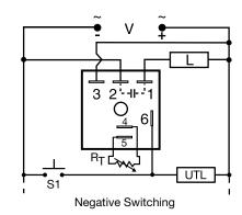
R<sub>T</sub> is used when external adjustment is ordered. Dashed lines are internal connections.
