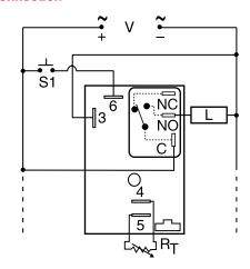
NO = Normally Open S1 = Initiate Switch L = Load C = Common, Transfer Contact
