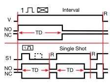
V = Voltage L = Load S1 = Initiate Switch TD = Time Delay R = Reset
