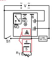
V = Voltage S1 = Initiate Switch C = Common, Transfer Contact NO = Normally Open NC = Normally Closed UTL = Untimed Load
