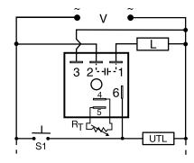
R<sub>+</sub> is used when external adjustment is ordered. Dashed lines are internal connections.
