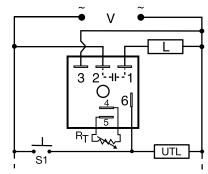
R<sub>x</sub> is used when external adjustment is ordered. Dashed lines are internal connections.
