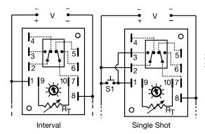
2-3 & 7-6 are Normally Open Contacts (NO) 2-4 & 7-5 are Normally Closed Contacts (NC)
