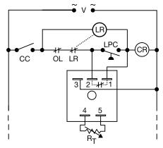
R<sub>T</sub> is used when external adjustment is ordered.
