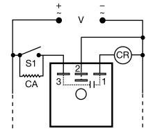
On initial closure of the S1, the compressor relay energizes immediately. When S1 opens or input voltage
