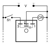
V = Voltage S1 = Initiate Switch CR = Compressor or Control Relay
