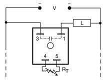
Load may be connected to terminals 3 or 1.  $R_{\!_{T}}$  is used when external adjustment is ordered.
