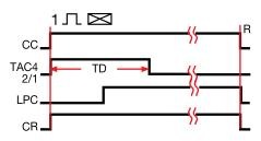
CC = Controller Contact CR = Compressor Relay LPC = Low Pressure Cutout
