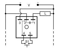
Internal connection between terminals 2 & 4. Dashed lines are internal connections.
