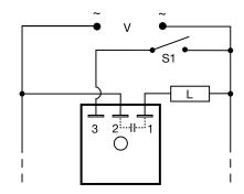
Note: Normally open output is shown. Normally closed output is also available.
