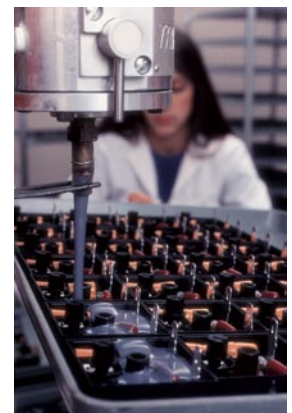
Each timing module and modular control is encapsulated for reliable, continuous operation.
