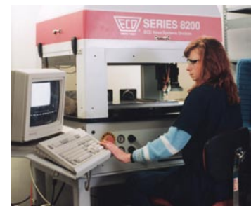
An operator inspects the automatic application of circuit board masking material.
