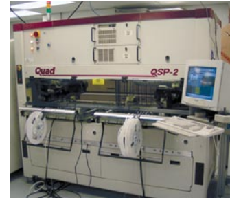
The second station places integrated circuits and microcontrollers.
