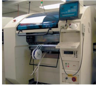
The first pick and place station places chip style surface mount components.
