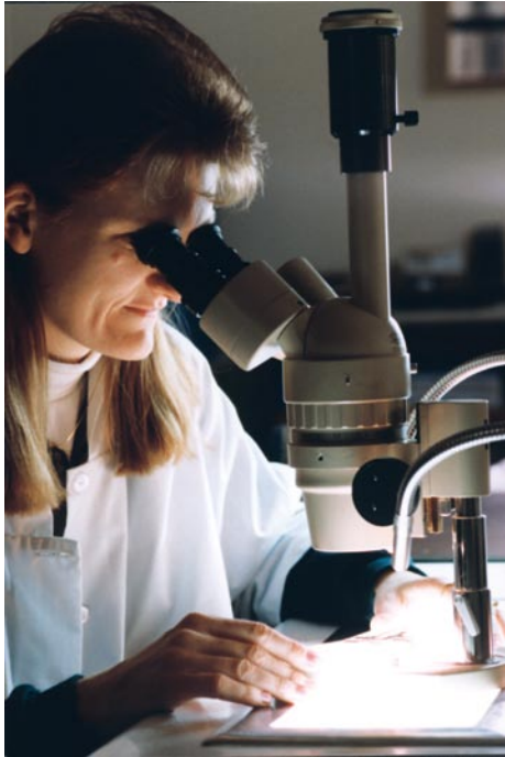
A Quality Control inspector carefully inspects printed circuit boards under a microscope to monitor material and vendor quality.
