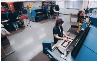
Automatic Insertion machines to insert: radial components, axial components, integrated circuits and terminals.
