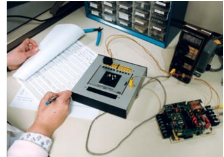
Individual components are tested to ensure that temperature specifications are not exceeded.
